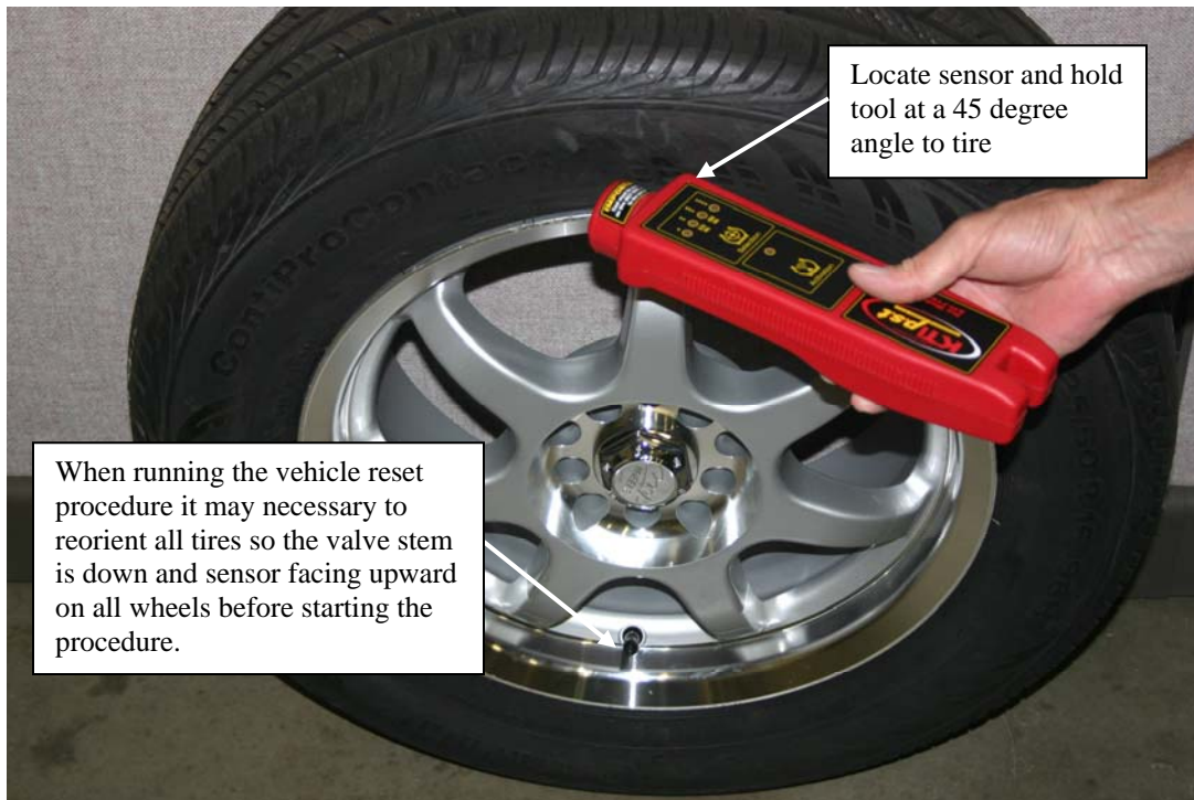
Figure 2 - PST Tool and Tire Orientation
